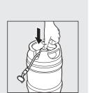
Simply open the lid and lft up the keg for approximately 5-10 seconds before setting back into the machine and closing the lid.
